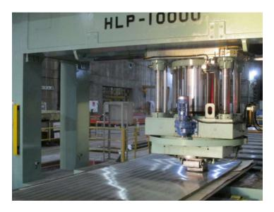
Press machine (corrects a plate using a hydraulic press and regulates flatness)
